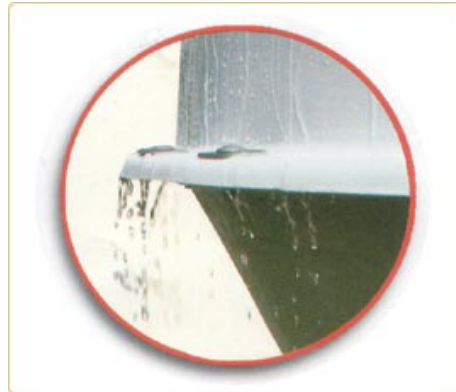
Inset showing water flowing over single joint and not flowing down cone into to feeder or barrow
